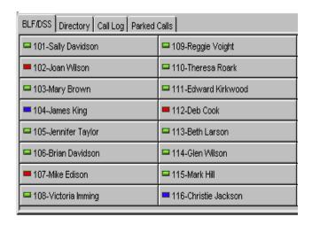
A green indicator on a BLF key signifies that the station is idle and can accept a call. When an indicator is red, the station is in use and cannot receive a call directly. The conditions which cause a station to be marked as in use include the telephone being offhook or the station being forwarded. The indicator is blue when the station has been set to do not disturb.
